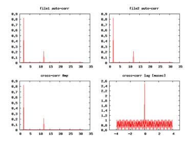
The plot shows the auto/cross-correlations for recorded track 8. The tone of 740 MHz (smaller peak) shows up at the expected position (channel 12). The large peak is an artifact that is due to the injected tone having too much power (around 20 dB above the noise). Due to time constraints the test could not be repeated with less tone power.
