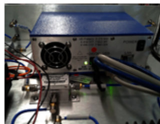
power LED on after fixing disconnected cable
