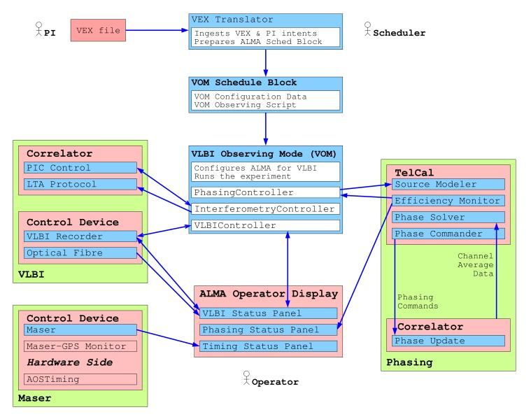
Modifications needed for ALMA software. The red boxes exist, the blue boxes have to be added for phasing ALMA, and the green colour groups boxes into larger units. (for details see attached paper)
