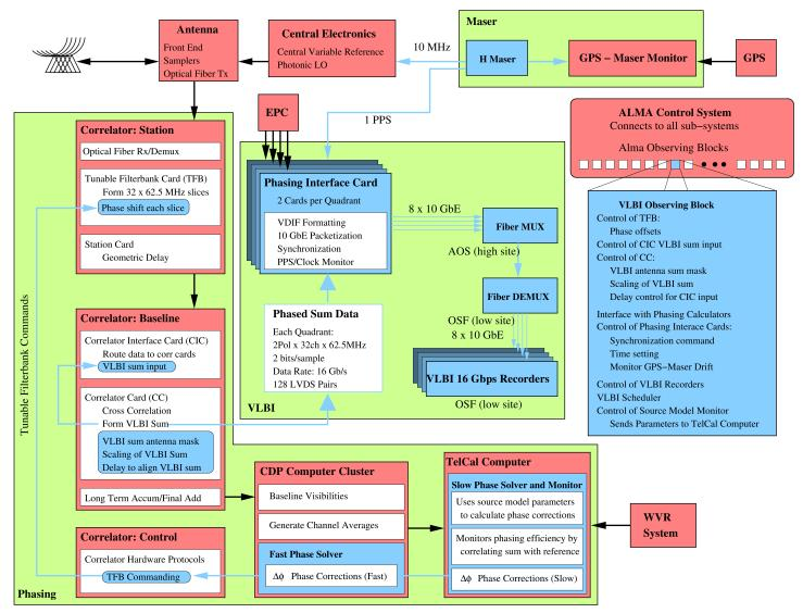
ALMA phasing block diagram. The red boxes exist, the blue boxes have to be added for phasing ALMA, and the green colour groups boxes into larger units. (for details see attached paper)
