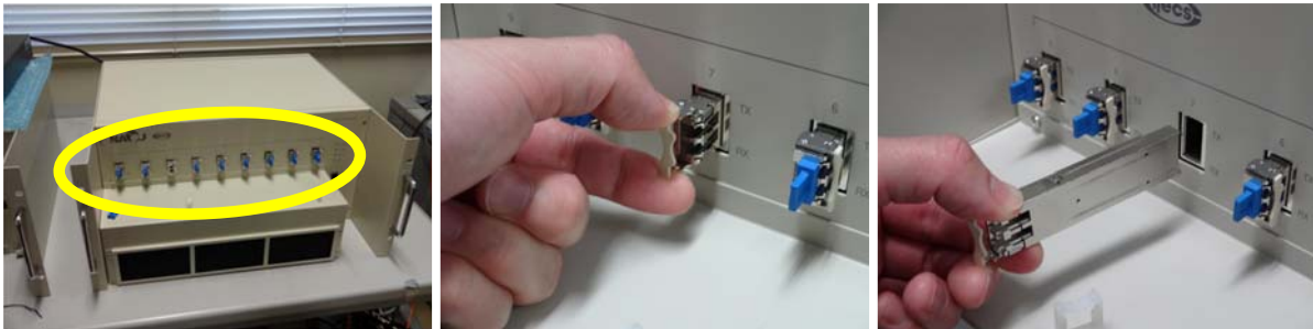
Figure 1: How to replace a 10GBASE-SR transceiver
