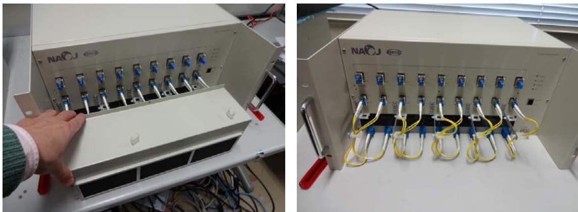
Figure 14: Pulling out the air filter box (left) and optical fibers (right)
