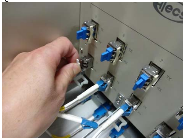
Figure 16: Pulling up the bale clasp before pulling out the ZR module.
