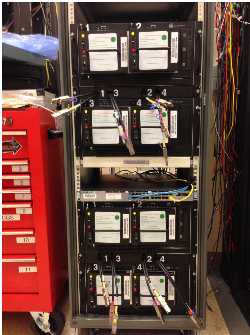
Figure 3.1: Recorder 1 and Recorder 4 housed in the test rack in the correlator lab. Note that each recorder consists of a host chassis (with slots 1 and 2) and an expansion chassis (with slots 3 and 4).
