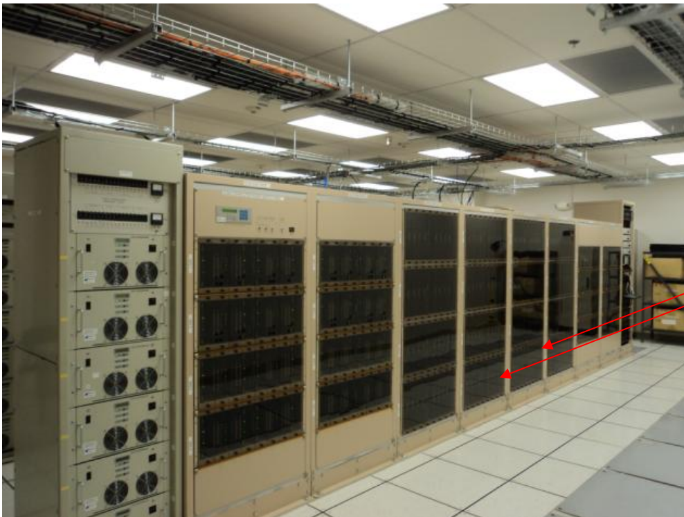
Figure 1: Photo of one correlator quadrant showing the selected locations for the PICs
