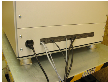
Figure 11: AC Power Connector & Cables Entry Point
