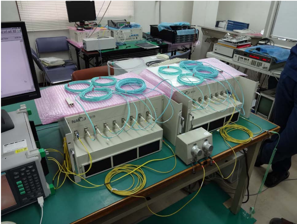
Figure 3-10: Photo of the Fiber Multiplexer and Fiber Demultiplexer during test
