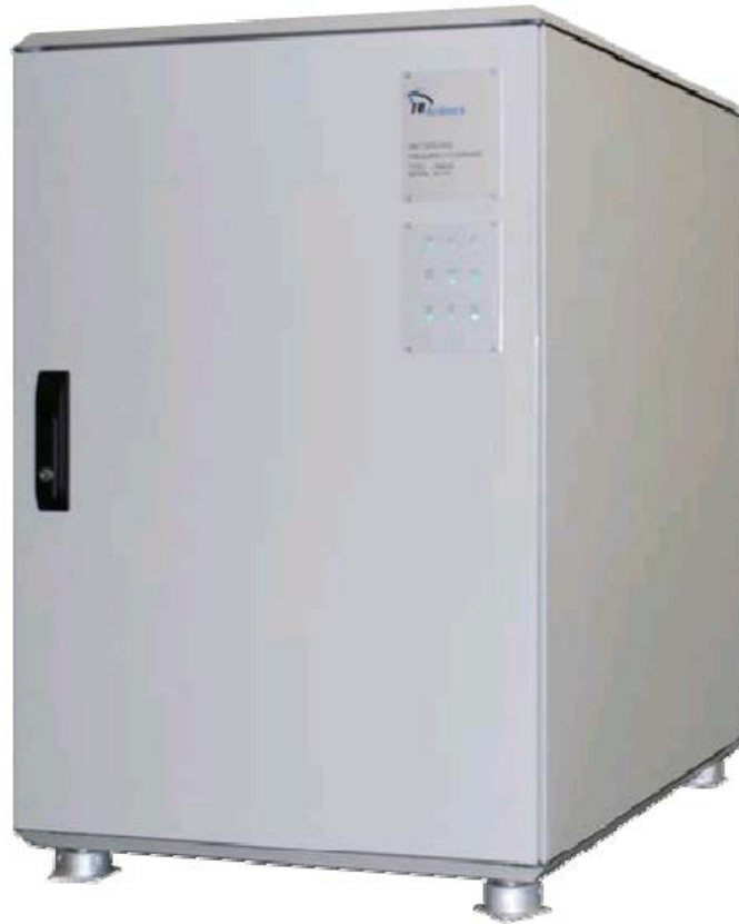
Figure 6 - Hydrogen Maser. Note: the maser assemblies are built into an RFI rack, which in turn will be mounted in a CLOA seismic rack.
