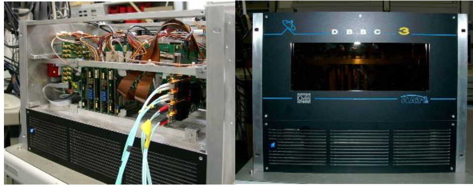
Fig. 5: Left: Internal view of the DBBC3. In the center the stack with the two ADB3-L and CORE3-L can be seen. Right: Front view of the DBBC3.
