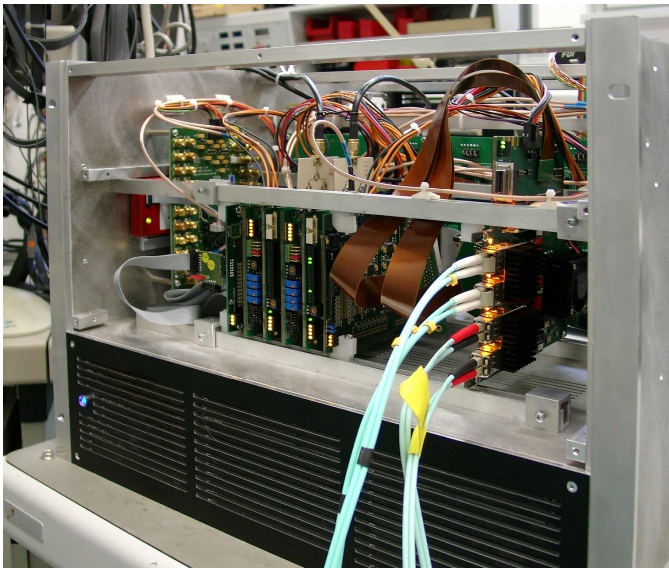
DBBC3L with CORE3L and FILA10G-S4
