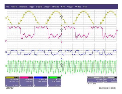
Figure 6: Example fo output converted signals, for an output tone at 4 MHz. From top: analog monitor, sign, magnitude, clock
