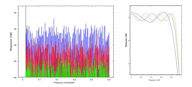
Figure 2: Stopband and passband response of prototype low-pass filter for 8 bit, 256 taps (blue), 9 bit, 384 taps (red) and 10 bit, 512 taps (green)
