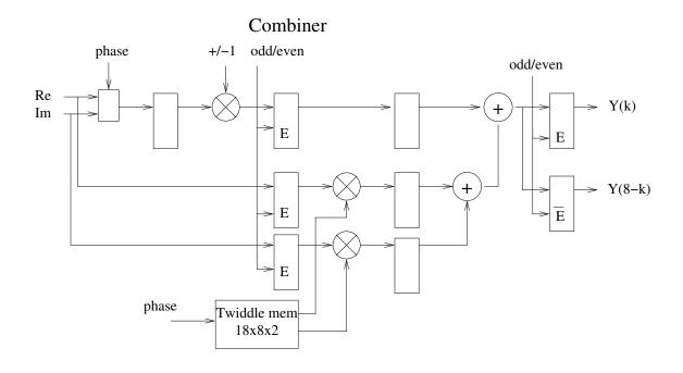
Figure 5: Structure of the conversion-to-real block
