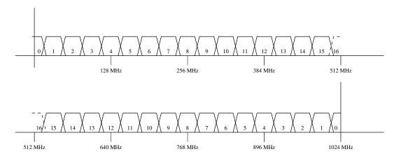
Figure 1: Conceptual description of the signal processing in the polyphase filterbank for an input signal in the  $1^{st}$  Nyquist range (0 to 512 MHz) and in the  $2^{nd}$  Nyquist range (512 to 1024 MHz)
